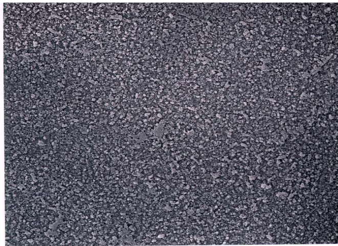
Figure 12 Electron Micrograph of RO Membrane Operated on Silica Laden Feedwater in the Presence of Product F
