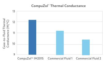
CompuZol IM2015 demonstrates significantly higher thermal conductance than other commercially available fluids.
