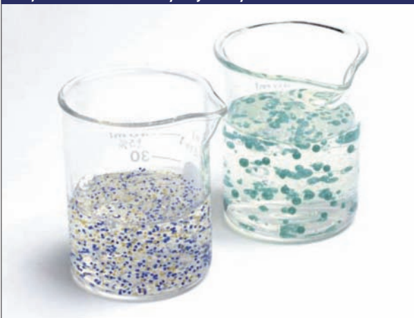
Figure 3. Acrylates Copolymer allows insoluble agents to be suspended without sacrificing clarity.
