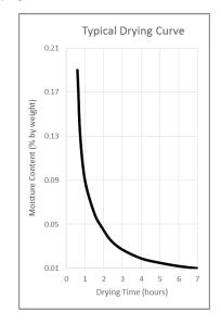
Figure 11. Typical drying curve for Pellethane® TPU
