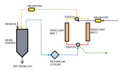
Figure 6. Schematic diagram of a two desiccant bed dryer.
