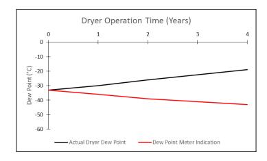
Figure 10. Example of the discrepancy between actual and measured dew point of dryer.
