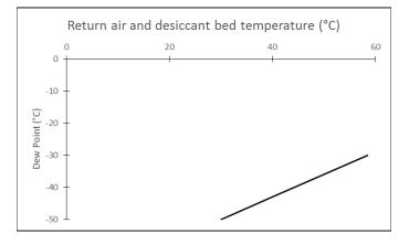
Figure 8. Dependency of dry air dew point on return air and desiccant bed temperature
