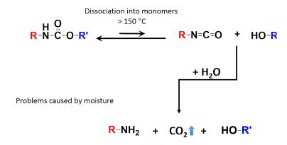
Figure 3. Result of moisture in TPU processing
