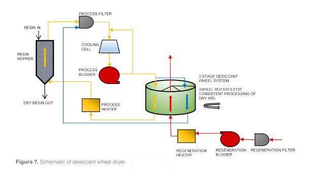
During operation of a desiccant bed dryer, the desiccant bed becomes saturated with moisture that has been removed from the resin. After a period of time, it becomes fully saturated and is no longer able to reduce moisture in the passing air. To further dry the material, the saturated desiccant bed first needs to release its absorbed moisture. The process of drying a desiccant bed is called "regeneration." This process is explained in detail in the "regeneration" section below.
