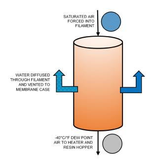
Figure 9. Diagram of membrane in compressed air/membrane dryer.
