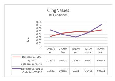
The third and most important property of the Release Lacquers is the release property itself, so, the level of blocking of the lacquer with the adhesive also called Cling. Cling must always be measured under different conditions to simulate different storage conditions, like tropical conditions, Normal testing would include cling tested at Standard conditions, 25°C and 50% humidity and Tropical conditions of 40°C and 90% humidity.
