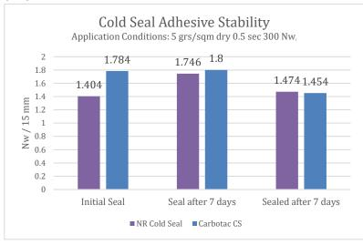
Control of the peel at low temperatures must be done as most of the products packaged using cold seal technology would be stored at freezing temperatures so care must be taken that the Cold Seal Adhesive does not loose bonds after storing at -5°C.
