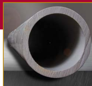
After years of service, the Corzan® pipe shows no sign of corrosion, scaling or degradation.
